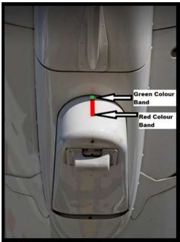
Normal Tail Skid without Damage
