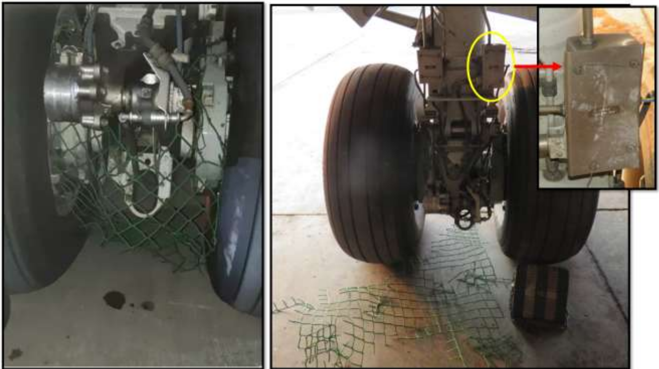
Mesh wire found entangled after landing at Mumbai
