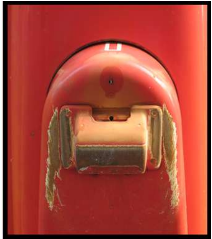
Damaged Tail Skid of the aircraft
