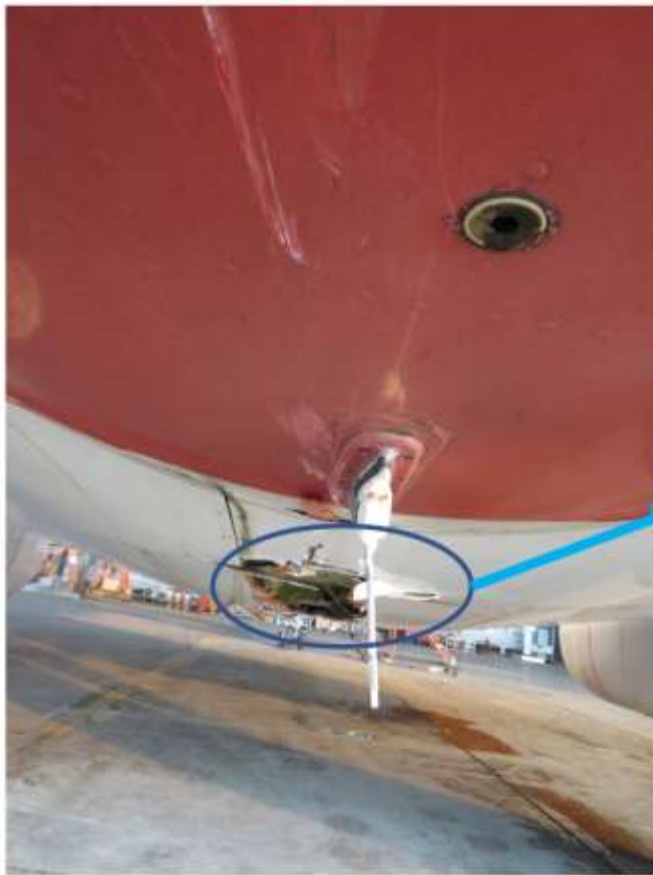
Detailed view of damages observed on Lower Fuselage Section (aircraft Belly)
