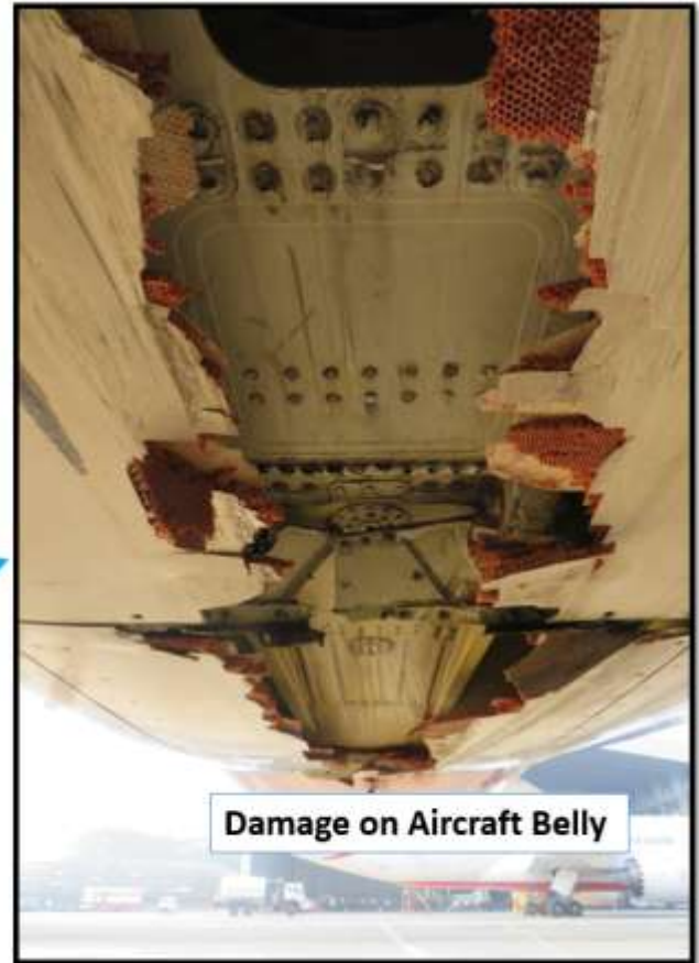
Detailed view of damages observed on Lower Fuselage Section (aircraft Belly)
