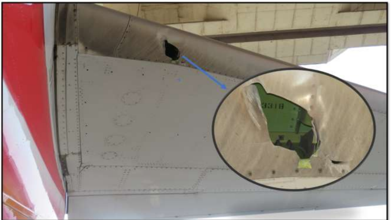
Damage on LH Horizontal Stabilizer
