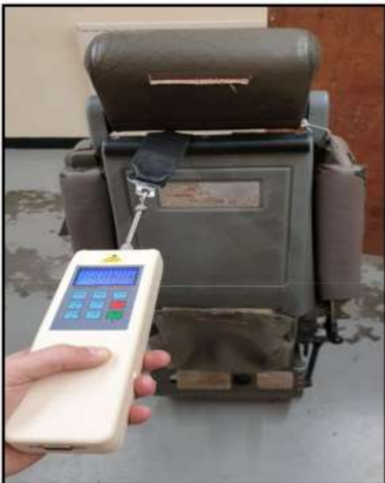
Measurement of Force required on Seat Recliner and Control Lever and Measurement of Force
