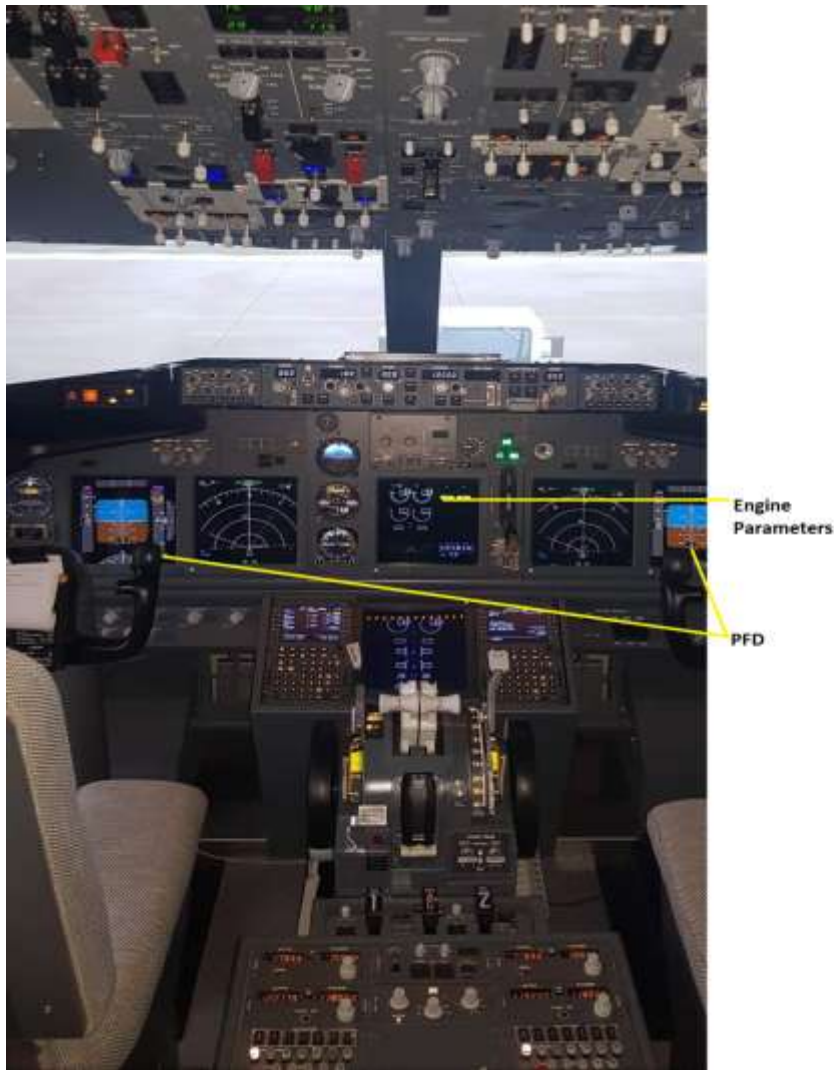
Cockpit Layout Boeing 737-800
