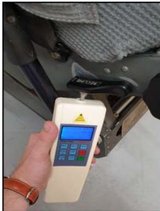
Measurement of Force required on Seat Recliner and Control Lever and Measurement of Force
