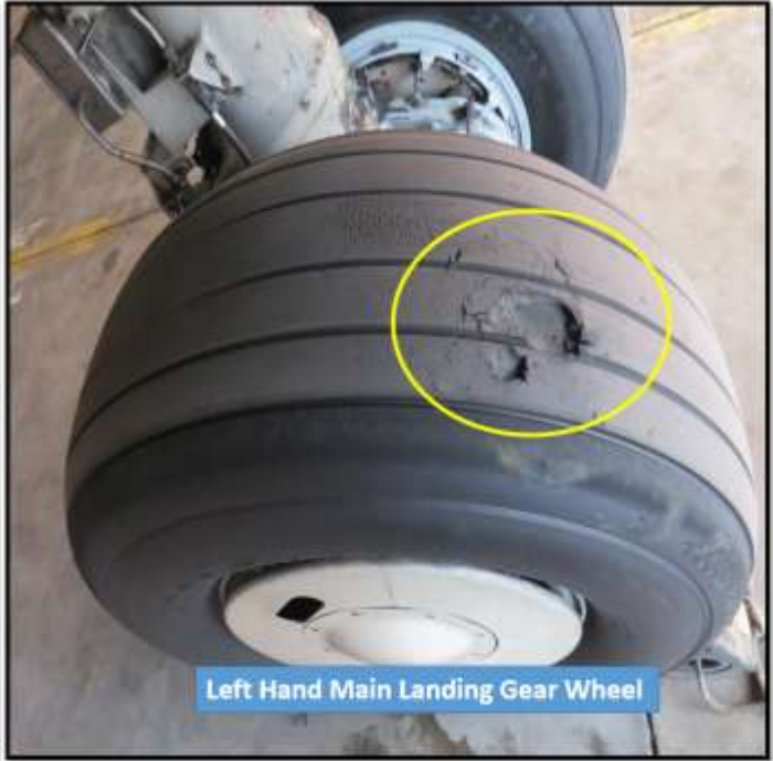
Damage on Lower Beacon & LH MLG Tyre
